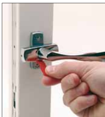
The cover plate is loosened and turned. The dismantling key ASSA 7339 is pushed into the slot on the handle plate.
